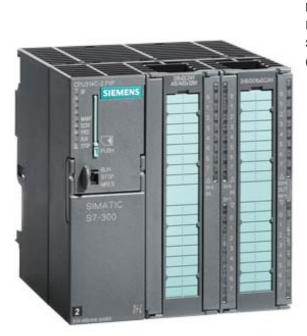
SIMATIC S7-300, CPU 314C-2 PTP COMPACT CPU WITH MPI, 24 DI/16 DO, 4AI, 2AO, 1 PT100, 4 FAST COUNTERS (60 KHZ), INTEGRATED INTERFACE RS485, INTEGRATED 24V DC POWER SUPPLY, 192 KBYTE WORKING MEMORY, FRONT CONNECTOR (2 X 40PIN) AND MICRO MEMORY CARD REQUIRED
