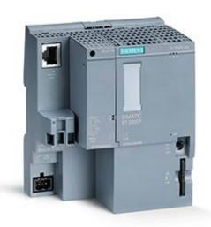
\*\*\*SPARE PART\*\*\* SIMATIC DP, CPU 1510SP-1 PN FOR ET 200SP, CENTRAL PROCESSING UNIT WITH WORKING MEMORY 100 KB FOR PROGRAM AND 750 KB FOR DATA, 1. INTERFACE, PROFINET IRT WITH 3 PORT SWITCH, 72 NS BIT-PERFORMANCE, SIMATIC MEMORY CARD NECESSARY, BUSADAPTER NECESSARY FOR PORT 1 AND 2
