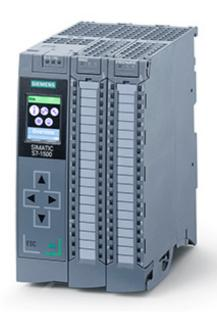
SIMATIC S7-1500 COMPACT CPU CPU 1511C-1PN, CENTRAL PROCESSING UNIT WITH WORKING MEMORY 175 KB FOR PROGRAM AND 1 MB FOR DATA, 16 DIGITAL INPUTS, 16 DIGITAL OUTPUTS, 5 ANALOG INPUTS, 2 ANALOG OUTPUTS, 6 HIGH SPEED COUNTERS, 4 HIGH SPEED COUNTERS FOR PTO/PWM/FREQUENZY OUTPUT 1. INTERFACE: PROFINET IRT WITH 2 PORT SWITCH, 60 NS BIT-PERFORMANCE, INCL. FRONT CONNECTOR PUSH-IN, SIMATIC MEMORY CARD NECESSARY
