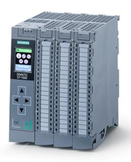
SIMATIC S7-1500 COMPACT CPU CPU 1512C-1 PN, CENTRAL PROCESSING UNIT WITH WORKING MEMORY 250 KB FOR PROGRAM AND 1 MB FOR DATA, 32 DIGITAL INPUTS, 32 DIGITAL OUTPUTS, 5 ANALOG INPUTS, 2 ANALOG OUTPUTS, 6 HIGH SPEED COUNTERS, 4 HIGH SPEED COUNTERS FOR PTO/PWM/FREQUENZY OUTPUT 1. INTERFACE: PROFINET IRT WITH 2 PORT SWITCH, 48 NS BIT-PERFORMANCE, INCL. FRONT CONNECTOR PUSH-IN, SIMATIC MEMORY CARD NECESSARY
