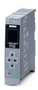
SIMATIC S7-1500F, CPU 1513F-1 PN, CENTRAL PROCESSING UNIT WITH WORKING MEMORY 450 KB FOR PROGRAM AND 1.5 MB FOR DATA, 1. INTERFACE: PROFINET IRT WITH 2 PORT SWITCH, 40 NS BIT-PERFORMANCE, SIMATIC MEMORY CARD NECESSARY
