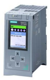
SIMATIC S7-1500, CPU 1515-2 PN, CENTRAL PROCESSING UNIT WITH WORKING MEMORY 500 KB FOR PROGRAM AND 3 MB FOR DATA, 1. INTERFACE: PROFINET IRT WITH 2 PORT SWITCH, 2. INTERFACE: PROFINET RT, 30 NS BIT-PERFORMANCE, SIMATIC MEMORY CARD NECESSARY
