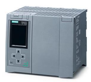
SIMATIC S7-1500F, CPU 1517F-3 PN/DP, CENTRAL PROCESSING UNIT WITH WORKING MEMORY 3 MB FOR PROGRAM AND 8 MB FOR DATA, 1. INTERFACE: PROFINET IRT WITH 2 PORT SWITCH, 2. INTERFACE: PROFINET RT, 3. INTERFACE: PROFIBUS, 2 NS BIT-PERFORMANCE, SIMATIC MEMORY CARD NECESSARY
