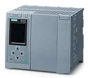
SIMATIC S7-1500F, CPU 1518F-4 PN/DP, CENTRAL PROCESSING UNIT WITH WORKING MEMORY 6 MB FOR PROGRAM AND 20 MB FOR DATA, 1. INTERFACE: PROFINET IRT WITH 2 PORT SWITCH, 2. INTERFACE: PROFINET RT, 3. INTERFACE: ETHERNET, 4. INTERFACE: PROFIBUS, 1 NS BIT-PERFORMANCE, SIMATIC MEMORY CARD NECESSARY
